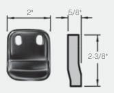
S459 Optional Rim Strike For Non Fire Rated 5100 Rim x Vertical Rod Device on a Pair of Doors without a Mullion. Black Powder Coated Investment Cast Stainless Steel.
