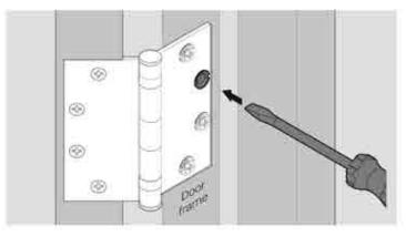
Determine which hinge needs adjustment to allow the door to hang properly in the door frame. Loosen but do not remove the screws from the hinge. For best results; only back out screws two turns.
