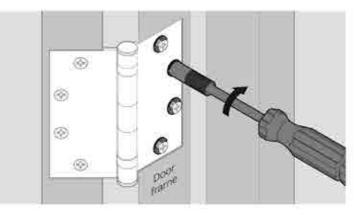
Insert screwdriver through adjustment tool. Slide adjustment tool down to position onto the quick shim adjustable collar and turn the collar to make appropriate adjustment. Once adjustment is complete, simply tighten the screws. Repeat if alignment needs further adjustment.
